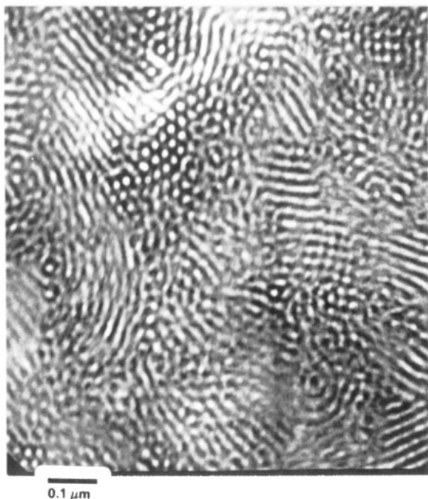
Figure 8. STEM photomicrograph of SBS block copolymer. Sample prepared by precipitation from solution then compression molding of precipitate. Thin sections exposed to OsO 4 vapor to yield dark rubber phase.
